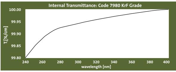
HPFS\* KrF Grade is certified to meet  $T_i \ge 99.8\%/cm@248nm$ , when measured through a polished, uncoated sample. A typical internal transmittance curve for HPFS\* KrF Grade fused silica is shown here.
