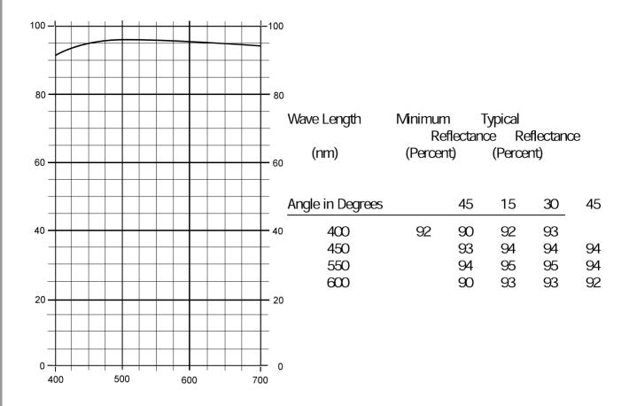
Enhanced aluminum mirrors are front surface mirrors overcoated with dielectric layers to increase reflectivity and protect against humidity and abrasion.
