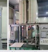
Chemical Tempering Machine(L)
